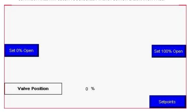
The 3R Valve Control Panel Valve Position Page allows the Operator the ability to calibrate the valve Linear Position Feedback from the Linear Potentiometer, "ZS-1".
