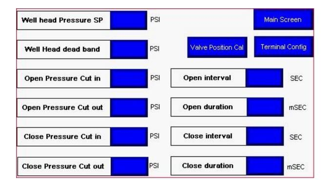
The 3R Valve Control Panel Setpoints Page allows the Operator the ability to enter system setpoints (Refer to P&ID for additional information):
