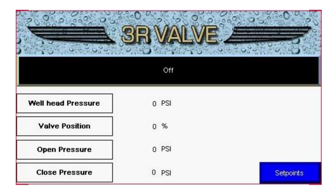
The 3R Valve Control Panel Main Page displays the following information;
